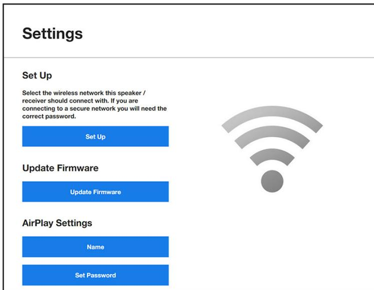
5. To manually setup the wireless Play-Fi receiver on a wireless network or to assign a static IP address click on "Set Up" and follow the on-screen instructions
